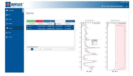
Geologist can view gamma logging data from the office, within minutes of completion of the gamma log, and make immediate decisions.
