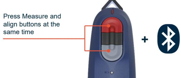
Turn on the device and enter the pairing mode by pressing the Measure (red) and Align (grey) buttons at the same time for approximately 5 seconds until the blue and green lights illuminate; and the red-light flashes.
