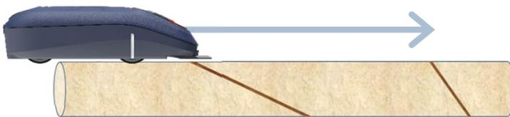
Roll the LOGRx device down the core along the orientation line (check that the depth increases in the software interface).
